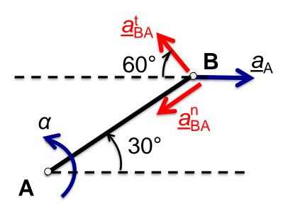
Calculate acceleration of B by resolving equation (2) in horizontal and vertical directions:
