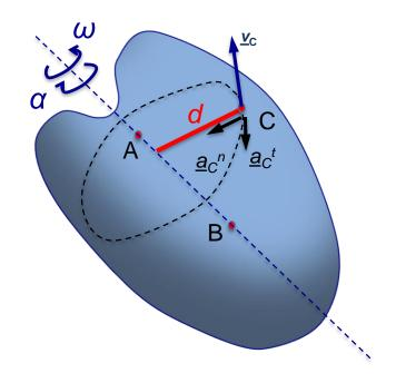
Kinematics of rigid body governed by: $\theta(t)$ angle of rotation $\dot{\theta}(t) = \omega(t)$ angular velocity $\ddot{\theta}(t) = \alpha(t)$ angular acceleration
